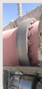
Kiln Outlet tyre shimming done
