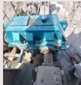
Cement mill 3 mill discharge bucket elevator 563BE1 gearbox changed
