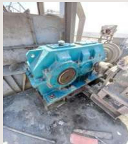
Cement mill 3 mill discharge bucket elevator 563BE1 gearbox changed
