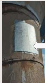
Cyclone casing crack
